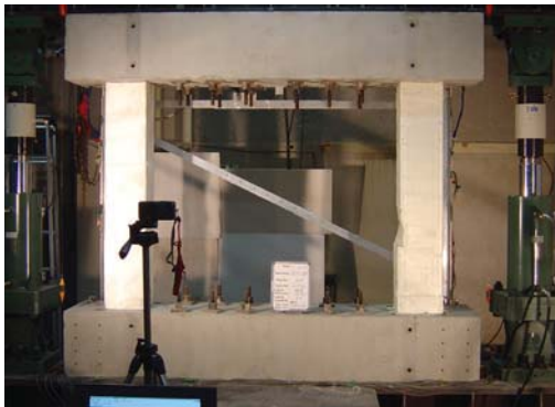
応急補強施工後
